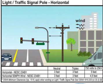
GUIDE FOR OPERATION OF EQUIPMENT NEAR POWER LINES
