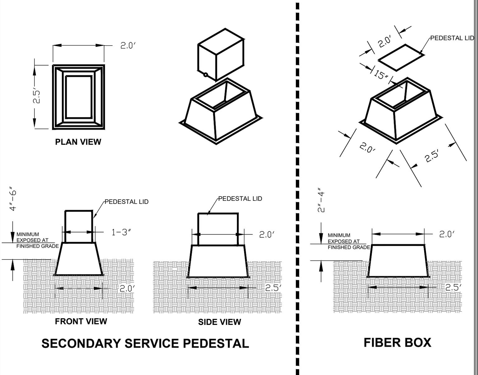
1. FIBER AND SECONDARY SERVICE PEDESTAL. BASE (GROUND SLEEVE) SHALL BE PROVIDED BY IDAHO FALLS POWER, BUT SHALL BE INSTALLED TO REQUIRED GRADE BY THE CONTRACTOR/DEVELOPER.
