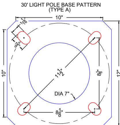
IF PRE-CAST CONCRETE LIGHT POLE IT SHALL MEET OR EXCEED ALL SPECIFICATIONS ABOVE
