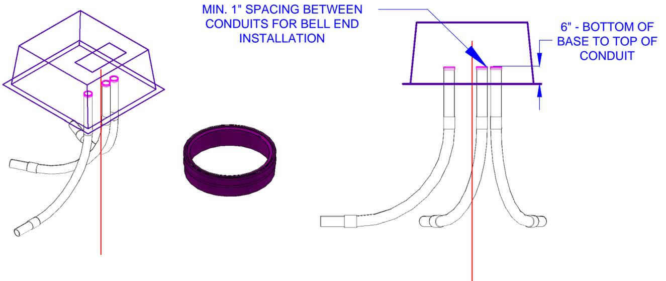
1. ALL CONDUIT (PRIMARY AND SECONDARY) MUST BE CUT TO 6" FROM BOTTOM OF BASE.
