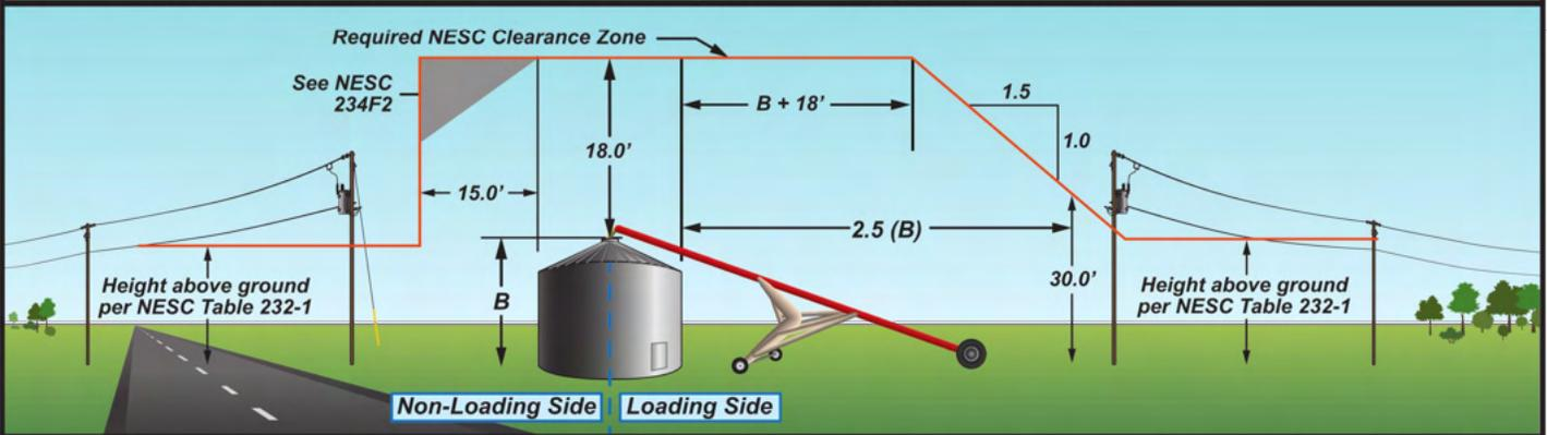
B = Vertical height to highest filling or probing port
